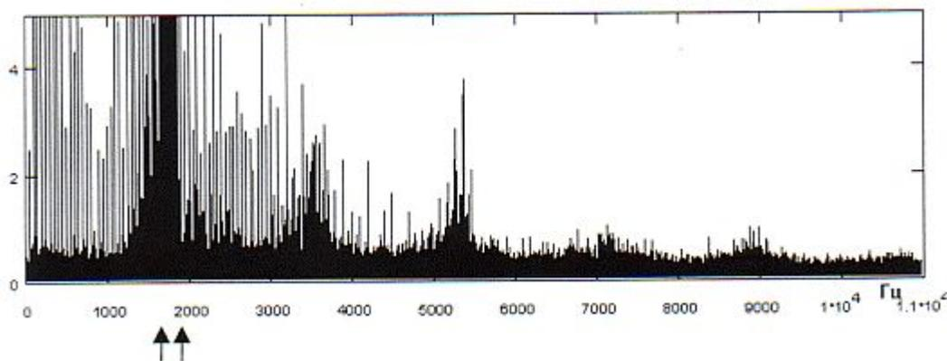
Fig. 2 the PLR-spectrum of a mineral (apofillit). Arrows (pointers) specify area of display of the spectrum, given in Fig. 2a.
