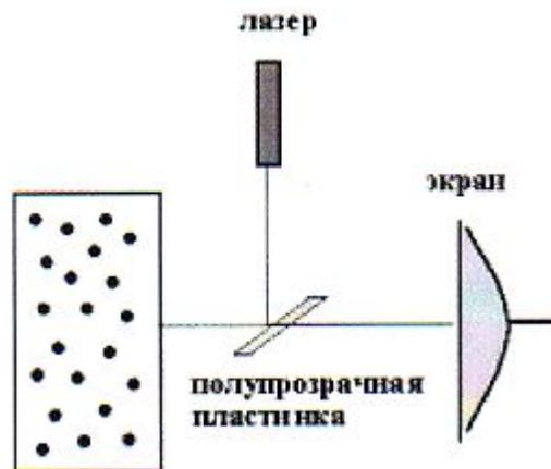
**Fig. 5 The scheme of experiment with supervision of weak localization of light**
